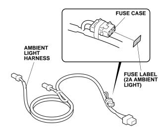
7. Plug the ambient light harness 12-pin connector into the driver's fuse box.
